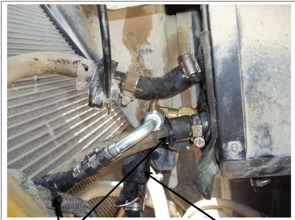
Picture shows all line connected. Note how the suction line fitting is completely tar taped to help insulate the expansion valve bulb. Put several layers of tar tape around the bulb area.
