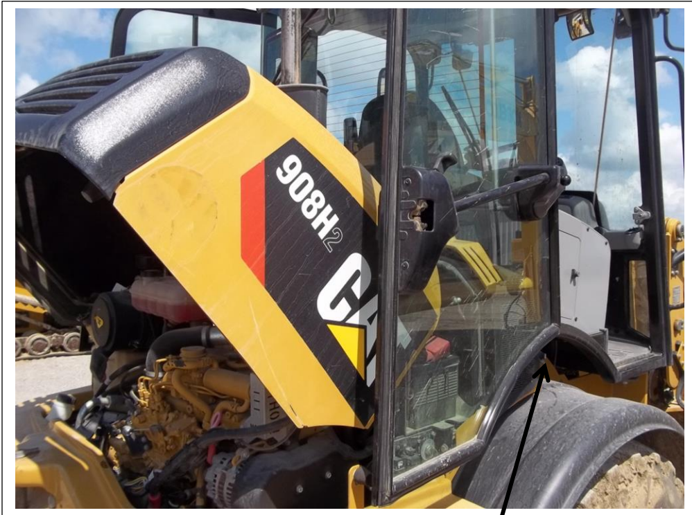
Remove this panel to get access to the heater hose connections. On the 906/908 H and H2 machines, remove the plastic fender first.
