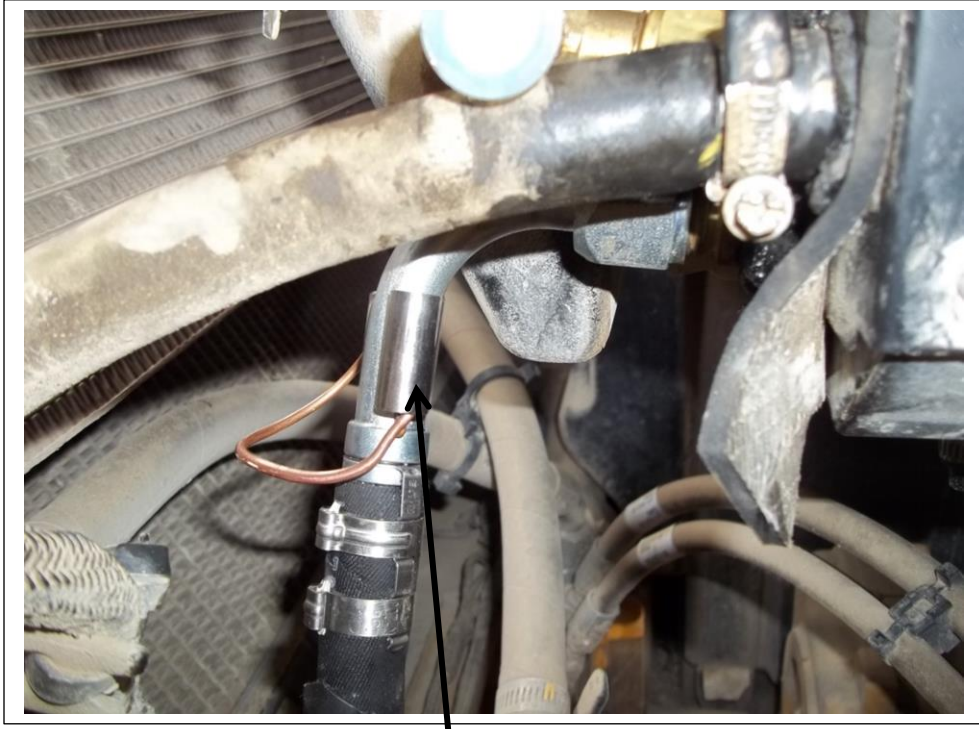
Expansion valve bulb clamp. Install as shown
